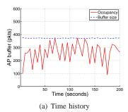
Fig. 9. Histories of buffer size and buffer occupancy with the eBDP algorithm when there are 10 downloads and no uploads.
